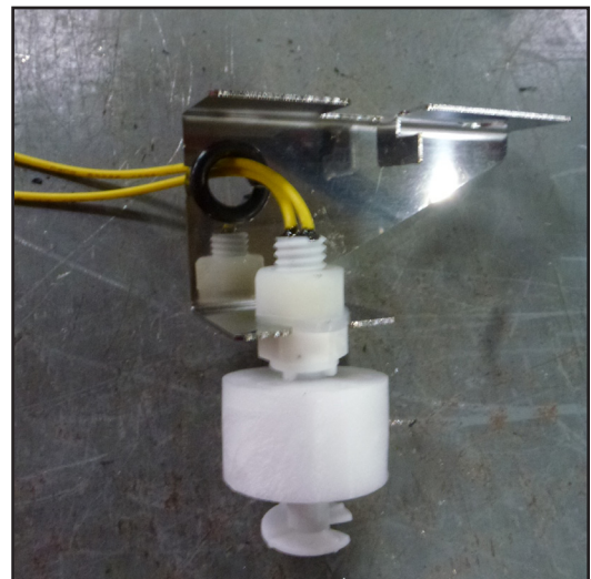
Figure 8: Picture of the float safety switch.
